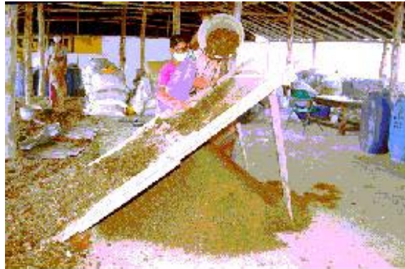
Fig. 6: Harvested compost being screened through mesh
