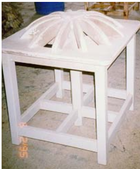
Photo 2: Dome type DODECA wooden frame for manual desalting
