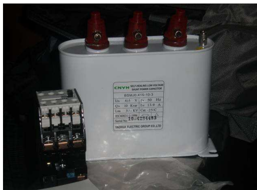
Figure 9. Capacitor's battery and contactor bought for the setting machine
